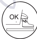
Mount the transducer parallel with the bottom.
