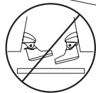
Mount the transducer parallel with the bottom.
